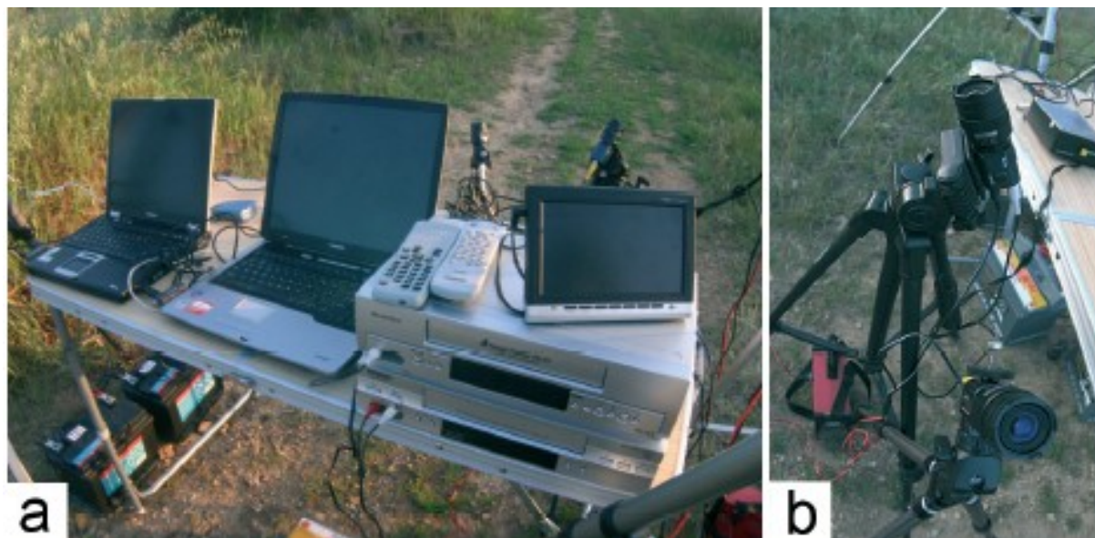
Fig. 3. A mobile SPMN recording station. a) System control table. b) Different sound and video detectors.
