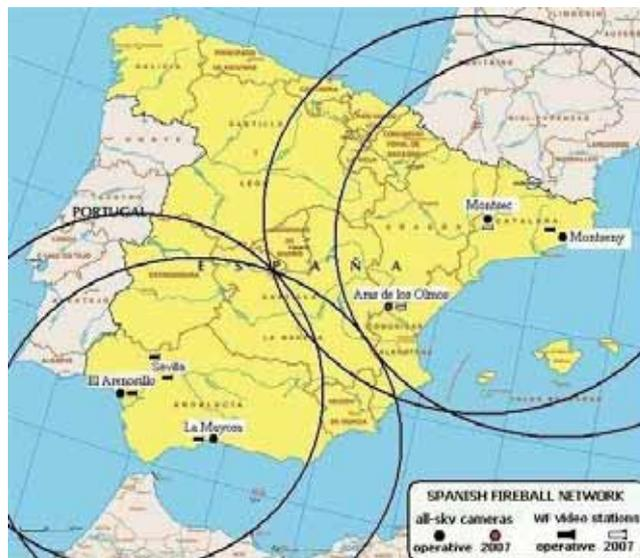
Figure 1 – Location of the SPMN all-sky stations. For image simplicity, only the names of the main stations are shown. The circles around the operative all-sky stations are the optimal range for bright fireball detection (350–400 km) although from some of the stations larger detection distances have been achieved (see e.g. Trigo-Rodríguez et al., 2003).
