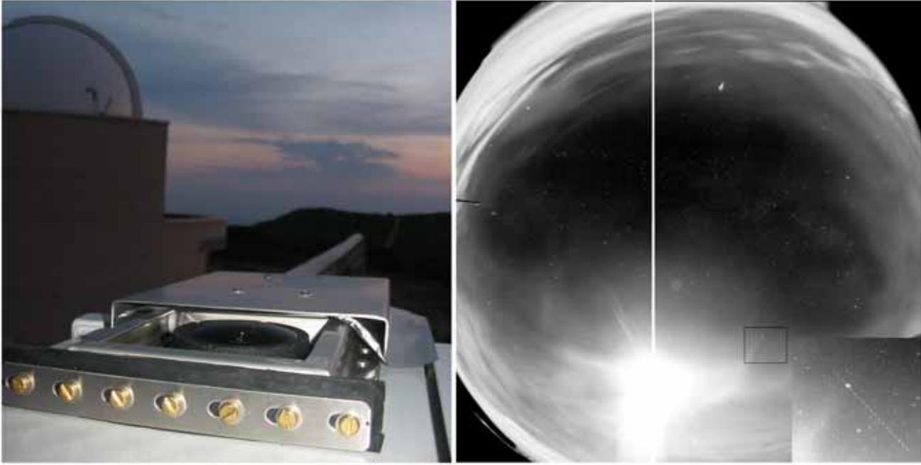
Figure 2 – An example of the excellent camera performance even under unfavourable conditions (partially cloudy skies with disturbing Moon). a) All-sky CCD camera of Montsec (SPMN station #3, OAdM). b) All sky-image taken by the camera shown in a). The black square nearby the full Moon includes an  $m = -2$  Perseid imaged on 2006 August 12.
